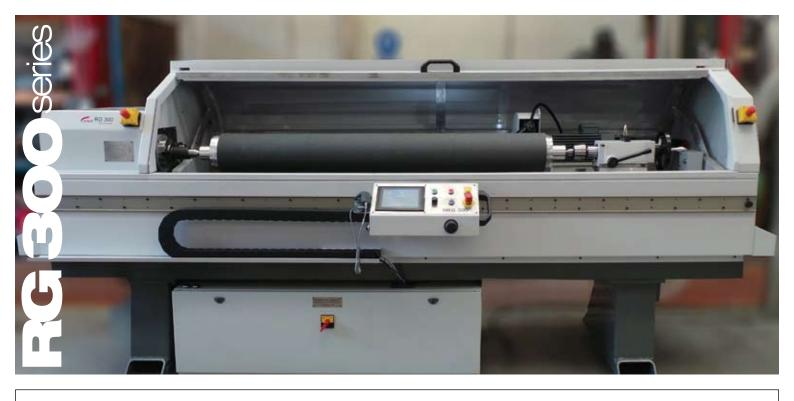
$RG300 \times 2000$  Maximum Diameter 300mm, Maximum Length 2000mm  $RG300 \times 3000$  Maximum Diameter 300mm, Maximum Length 3000mm
